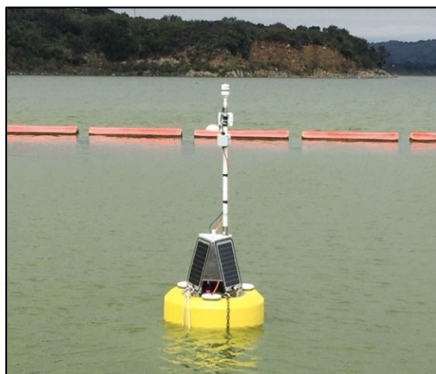
Lake Cachuma Water Quality Monitoring Buoy
