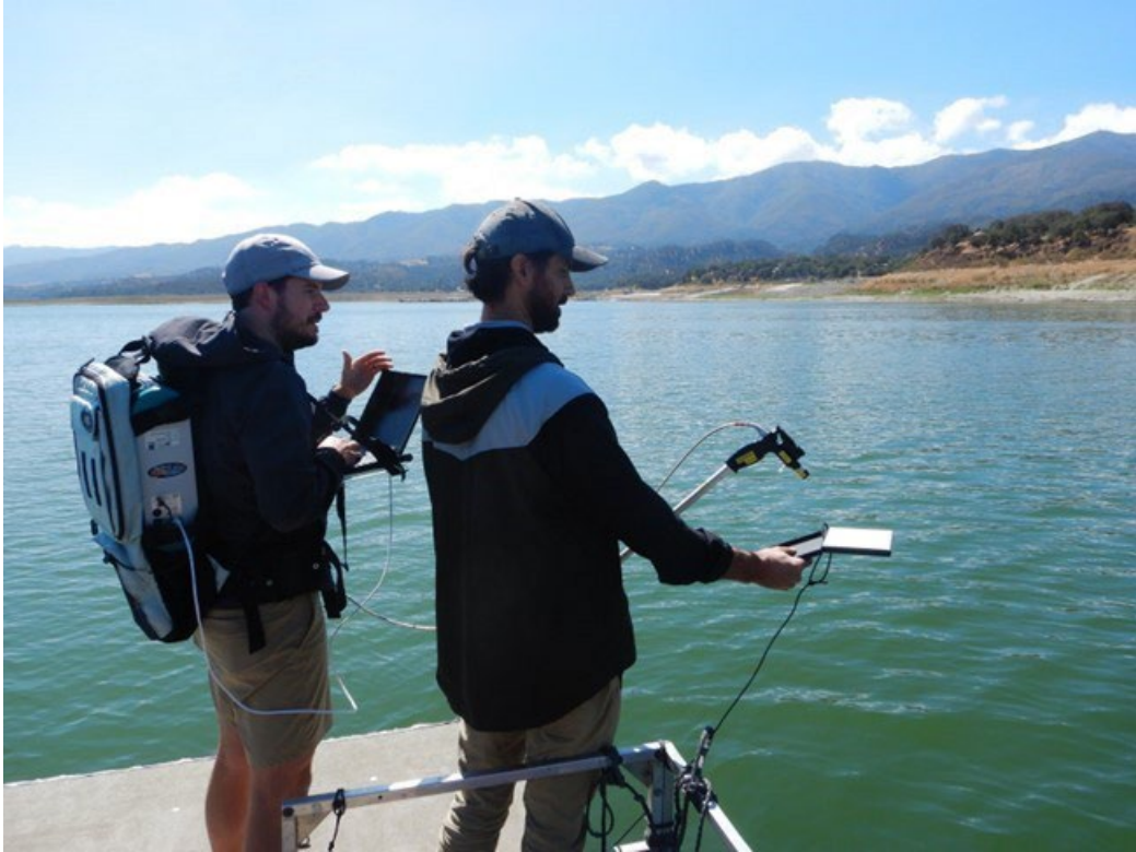
Figure 137: COMB staff assisting JPL staff with taking spectral reflectance and water quality data at Lake Cachuma during the AVIRIS overflight.
